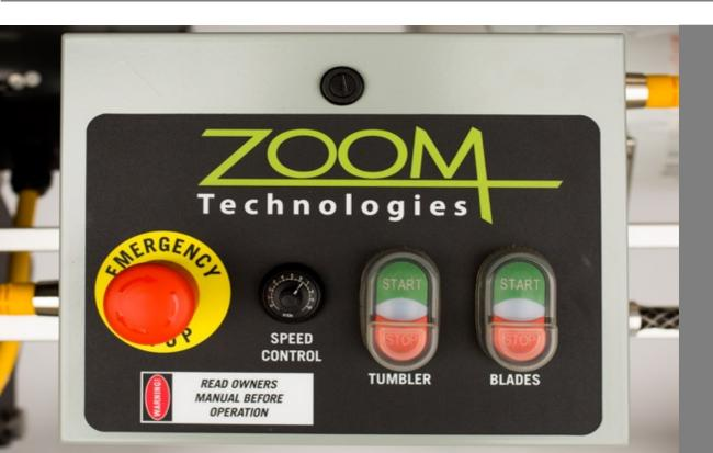
**Modularized Control Box with Tumbler Speed Control**
