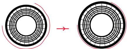
As soon as full contact between drum and shear band is achieved, release the tension knob.
